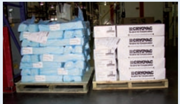
Vacuum-packed cheese pouches (left) compared with traditional carton packs. Vacuum-packing has allowed 140% more bags to be packed on a single pallet.
