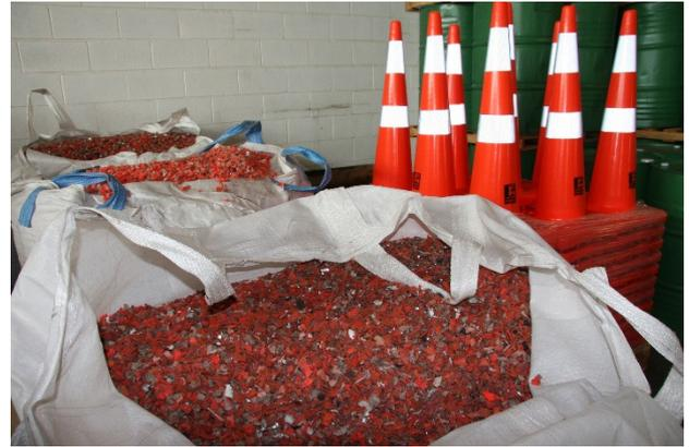
3. Granulated recycled material alongside new cones at the Proline factory
