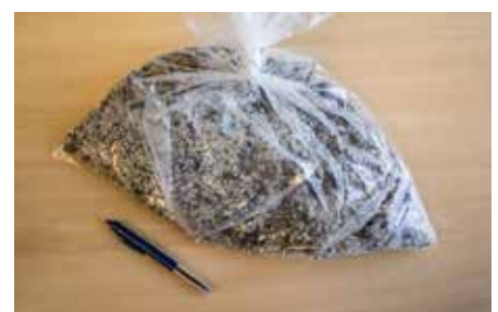
1.5kg of pellets collected in just 6 weeks from a LittaTrap™ filter device at a small NZ plastic manufacturing site
